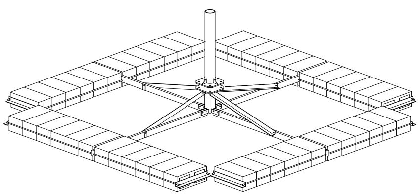
Shown with 12 block/leg ballast holders 8"x8"x16"nom. block supplied by customer
