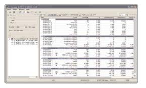
A MPEG-2 Transport Stream analyzer for real-time analyzing, monitoring and decoding for VENTUS 1.0. The T-SCOPE is compatible with ATSC, DVB-C, DVB-S, DVB-T and OpenCable modulations. T-SCOPE is the best solution for OEM manufacturers who seek the best of the best for designing and verifying digital TV equipment.
