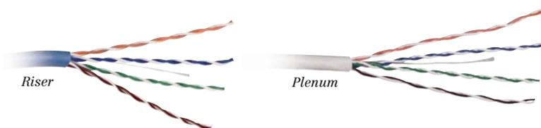
DataTwist 1200 Cable Series consists of 4-pair UTP cables that exceed the Category 5e requirements as per ANSI/TIA/EIA-568-B.2 standard. When used as the horizontal cable in the Belden IBDN System 1200, the channel provides 160 MHz of bandwidth and a data-rate of up to 1.2 Gb/s.
