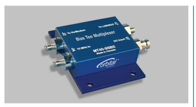
The Orbital Research "Mux-Tee" (MT-25/40) is a premium bias tee multiplexer that does much more than insert DC current: it multiplexes a 10 MHz reference signal onto the L-band signal. And because it is a passive device that requires no power, it can work in reverse and extract a DC signal and/or demultiplex a 10 MHz reference from your modem.
