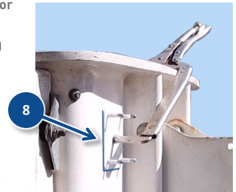
Figure 3: Fasten Tracker bracket glued and C-clamped to bucket.
