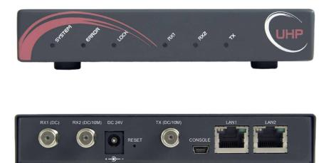
UHP Dual Gateway<sup>™</sup> provides optimum solution for hierarchical networks and makes it possible to design such networks with singlehop connectivity using low-cost VSAT terminals and affordable Regional Gateways (RGW). The Central Gateway (CGW) has a UHP TDM/TDMA Hub with at least one DVB carrier (TDM) and several TDMA return carriers. The Regional Gateway (RGW) also transmits a DVB (TDM) carrier and is capable of receiving one or more TDMA carriers.
