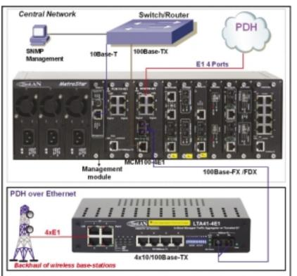
The MMM-01 Management module installed in the MetroStar System will monitor, control and manage the modules in the MetroStar chassis and the remote LTA41-XE1 or T1
