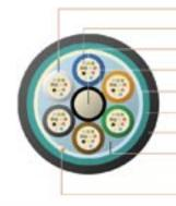
Gel-Free Buffer Tube **Optical Fibers** Central Member Central Member Jacket **Dielectric Strength Elements** Corrugated Steel Armor **Outer MDPE Jacket** DryBlock<sup>®</sup> Water-Blocking Material
