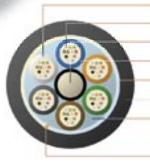
Gel-Free Buffer Tube Optical Fibers Central Member Central Member Jacket Dielectric Strength Elements Outer PE Jacket DryBlock<sup>®</sup> Water-Blocking Material
