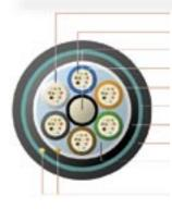
Gel-Free Buffer Tube **Optical Fibers** Central Member Central Member Jacket **Dielectric Strength Elements Corrugated Steel Armor** Inner MDPE Jacket Outer MDPE Jacket DryBlock® Water-Blocking Material Ripcord
