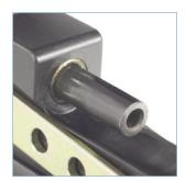
set at the factory and requires no field calibration. Each tool is clearly marked with a .710 or .830 to quickly indicate the fixed setting dimension.
