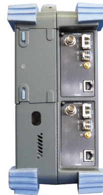
The FTB-8525/8535 Packet Blazer modules are also compatible with the FTB-400 Universal Test System and FTB-500 Platform. Here, two FTB-8535 modules are shown in the FTB-400, addressing multichannel applications.
