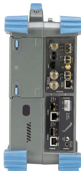
The FTB-8510B Packet Blazer Ethernet Test Module is also compatible with the FTB-400 Universal Test System and FTB-500 Platform. Shown in the FTB-400, are the FTB-8510G Packet Blazer 10 Gigabit Ethernet Test Module and the FTB-8130 Transport Blazer Next-Generation SONET/SDH Test Module.
